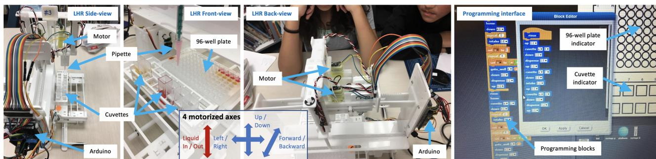
Figure 1: Liquid Handling Robot (LHR) hardware and programming environment.
